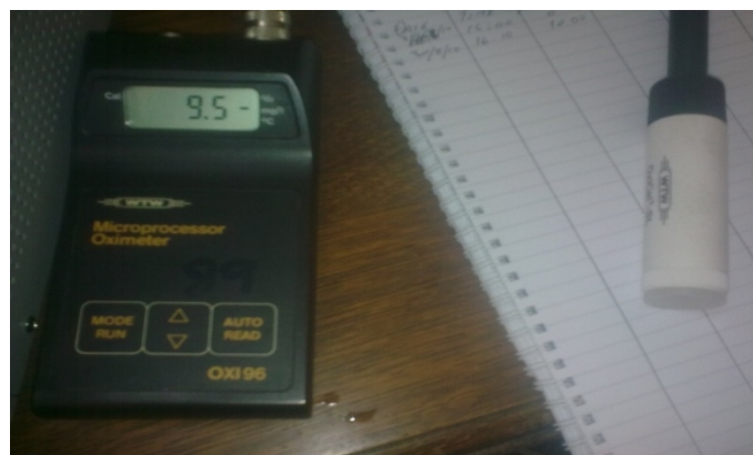
Figure 5 WTW Oxi 96 DO Meter.
